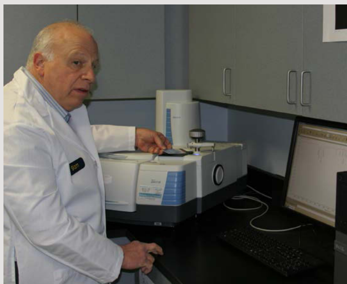
Analyst Sam Blittman discussing the proper use of the FTIR Instrument in Identifying Pure Organic Compounds
