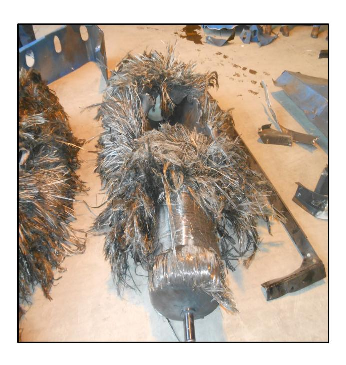
The two cylinders that exploded. Both failed near the middle of the tanks, it is presumed in the area of flame impingement.
