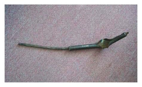
(2) Complete view of the first gas spring that exploded. The rod is still in place and the threads intact on both ends. Did this force the stairs downward, as reported by first in firefighters? If springs held up the pull-down stairs, heat may have caused them to lengthen and sag. This one remained in place (attached by one end) and was removed by the fire inspector from the damaged pull down stairs.
