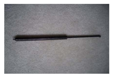
(3) The second cylinder rocketed and imbedded in the wall. The cylinder, the piston rod, and the threaded connections at each end are all intact. The rod moves freely, without resistance, for the length of the throw of the cylinder, but it feels as if the seal at the end of the rod inside the cylinder was damaged and no longer sealed.
