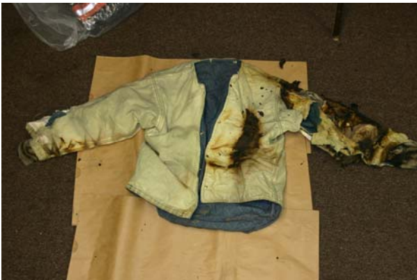
Thermal liner and moisture barrier (inside) of Firefighter 1's bunker coat
