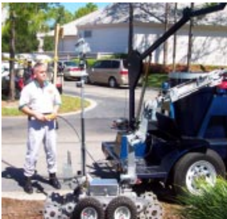
Investigator Spano using the robot to place a dummy pipe bomb in the bomb disposal trailer.
